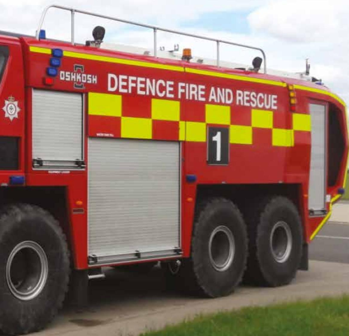
The new Oshkosh Striker which has a High Reach Extendable Turret (HERT) will gradually replace the MFV for the Defence Fire Services. At the moment the first few have been delivered to RAF Waddington, RAF Brize Norton, RAF Northolt and MOD Corsham to support initial training before they become operational in September 2020. This has been a special build for the MOD being narrower and having a smaller wheelbase to enable them to fit into existing fire stations.
