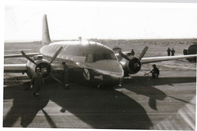
When this Viking of Eagle Airways took off from Bengazi it had a problem with its undercarriage. It still came to us and did a wheel's up landing on the Sand strip without catching fire. In the second picture you can see a DP1 and one of the lads putting his gloves on.
