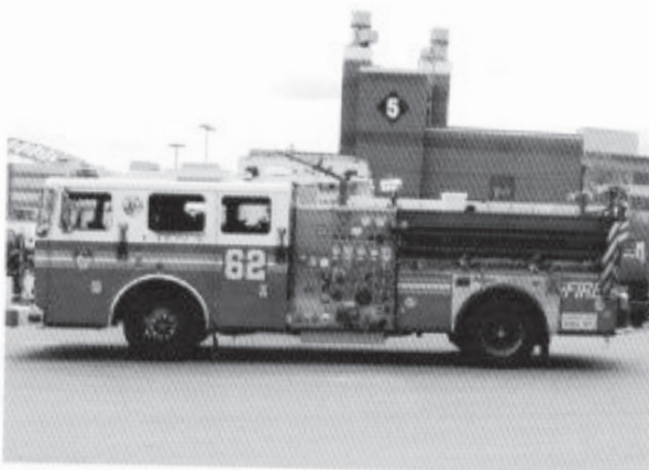
A view of the side pump
