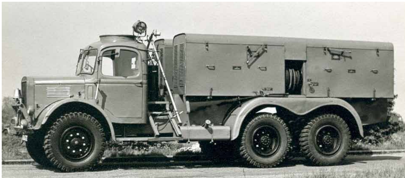
THE GAS TRUCK-Austin K6 6x4 CO 2 Tender
