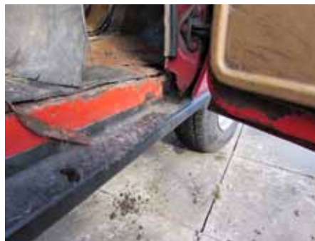
Inner and outer cills gone drivers side
